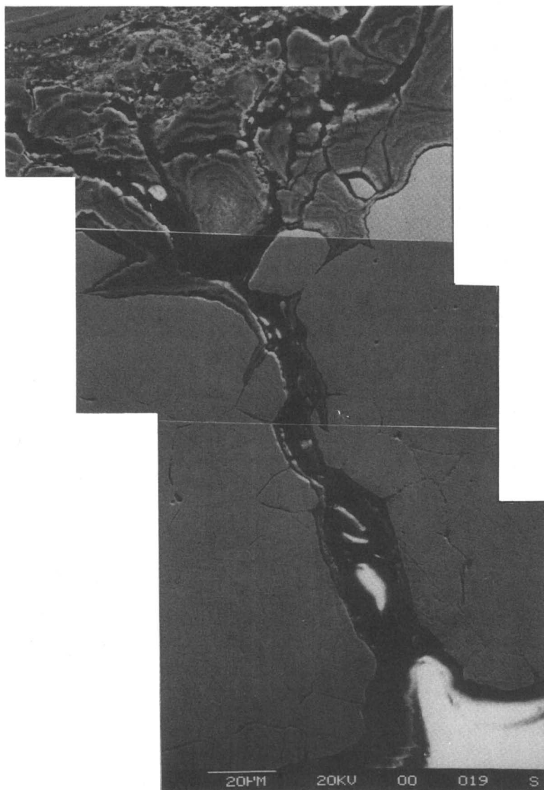
Figure 5. Cross-section of the a Hastelloy C-276 PFR preheater tube, which failed during experiments employing methylene chloride.
